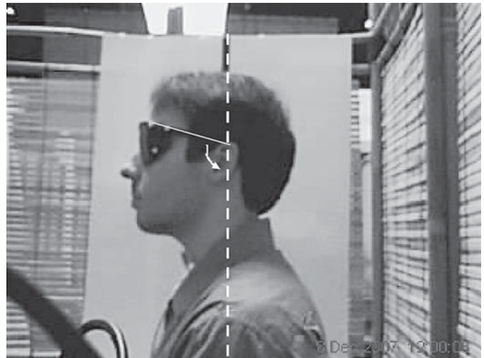
Fig. 1. A participant wearing goggles with yellow fluorescent markers allowing the extraction of head angle relative to the vertical axis of the image.
